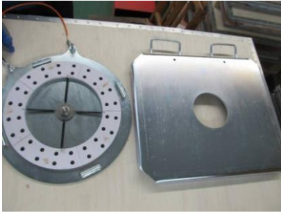
(Two-part Disassembly of Steel Plate Turntable)
